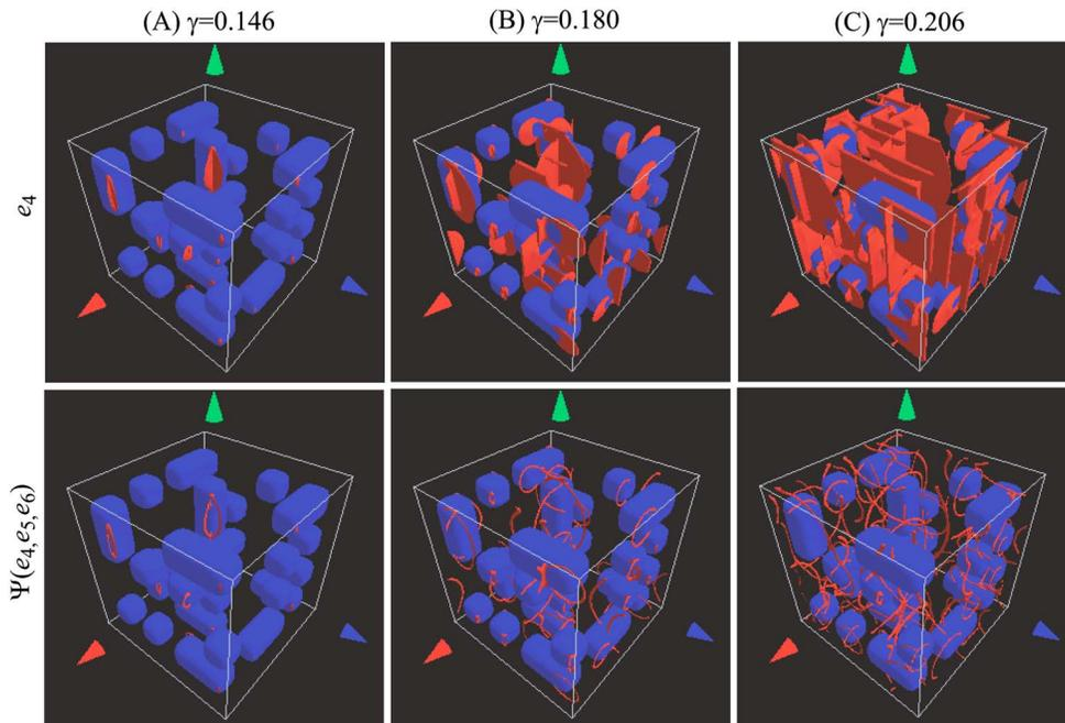
FIG. 3. (Color online) Time evolution of  $e_4$  (upper figures) and  $\Psi$  (lower figures) under shear  $\gamma = \dot{\gamma}t$ . They take large values on slip planes and dislocation cores, respectively. Blue regions represent hard domains. Dislocation loops are trapped at the interfaces.
