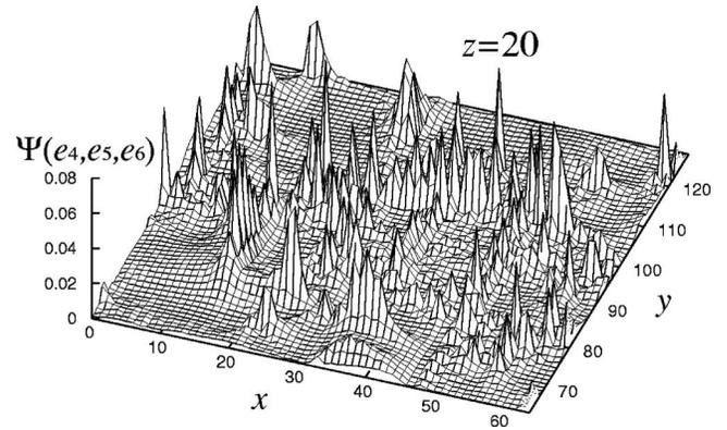
FIG. 2. (Color online) Shear strain  $e_4$  exhibiting slip planes (upper plate) and shear deformation energy  $\Psi$  at  $z=20$  with peaks at dislocation cores (lower plate) in a one phase state at  $\gamma=0.296$ . A 1/4 of the total plane is shown in the lower figure. The  $x$ ,  $y$ , and  $z$  axes are in red, blue, and green, respectively.
