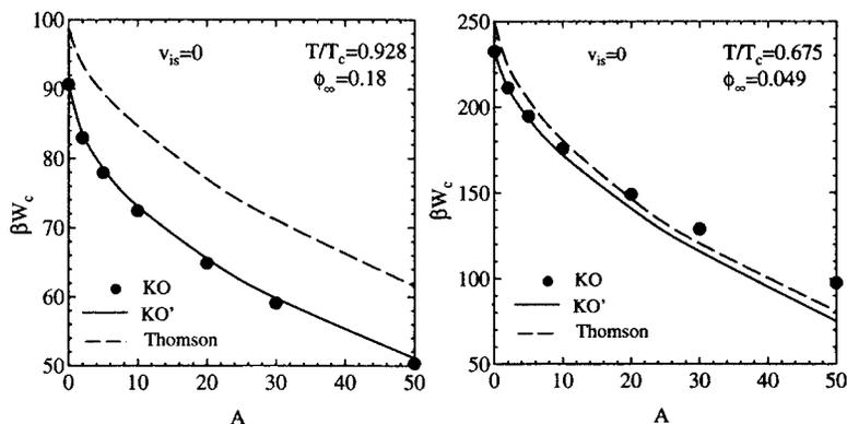
FIG. 9. Normalized free energy  $\beta W_c$  without  $v_{\text{is}}$  at  $T/T_c = 0.928$  (left) and  $0.675$  (right) as a function of  $A$ . The dots (●) (KO) are obtained by solving Eq. (2.21). The solid line (KO') is calculated from Eq. (3.14), while the broken line (Thomson) is from the first line of Eq. (3.16).
