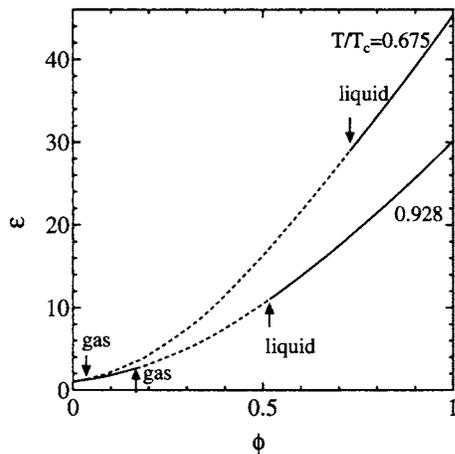
FIG. 1. Static dielectric constant  $\epsilon$  as a function of  $\phi = v_0 n$  at  $T/T_c = 0.675$  and  $0.928$  on the basis of the Harris-Alder formula (2.7) using the data water in Ref. 17. The dotted part corresponds to the two-phase region in the van der Waals model and is given by  $0.0358 < \phi < 0.729$  for  $T/T_c = 0.675$  and by  $0.168 < \phi < 0.519$  for  $T/T_c = 0.928$ .
