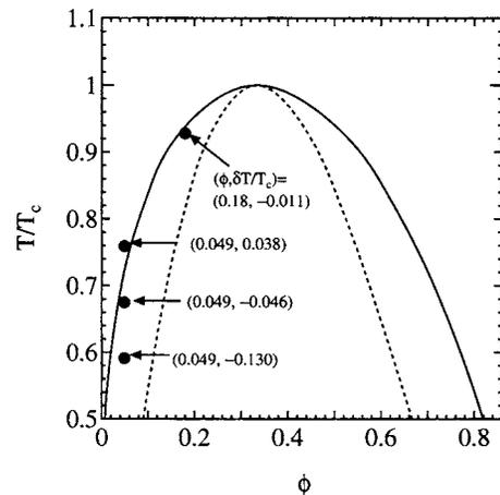
FIG. 2. Phase diagram in the plane of  $T/T_c$  and  $\phi = v_0 n$  with coexistence curve (solid line) and spinodal curve (dotted line). Use is made of the van der Waals model. At the dots (●) numerical calculations are performed in this work.
