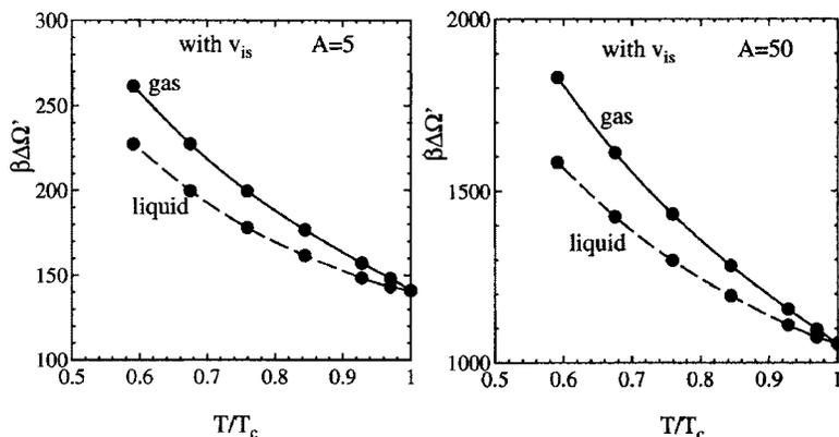
FIG. 5. Normalized solvation free energy  $\beta\Delta\Omega'$  with  $v_{is}$  around an ion for gas and liquid on the coexistence curve for  $A=5$  (left) and 50 (right).
