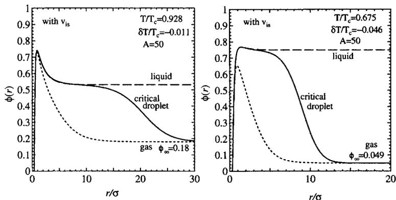
FIG. 7. Normalized density  $\phi(r)$  around an ion with  $A=50$  in a metastable gas with  $\phi_\infty=0.18$  (dotted line) and in the corresponding liquid (broken line) at  $T/T_c=0.928$  (left) and 0.675 (right). Also shown is the critical droplet obtained from Eq. (2.19). Here  $u_{\text{is}}$  is present and  $n(r)$  tends to zero at small  $r$ .
