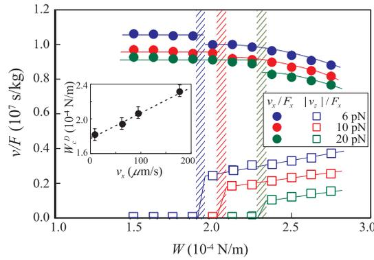
**Figure 5.** Dependence of the particle mobility both parallel and perpendicular to the field on the anchoring strength  $W$  and the driving force  $F_x$ . The inset shows the relationship between  $W_c^D$  and  $v_x$ .
