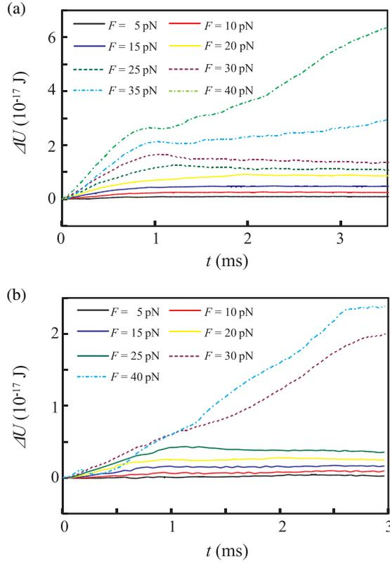
**Figure 2.** Time evolution of the stored elastic energy for various strengths of the applied force. (a)  $\mathbf{E} \parallel \mathbf{F}$  and (b)  $\mathbf{E} \perp \mathbf{F}$ . The solid, dashed, and chain-dashed lines correspond to figures 1(b) and (c), (d) and (e) for  $\mathbf{E} \parallel \mathbf{F}$  and (f) and (g), (h) and (i) for  $\mathbf{E} \perp \mathbf{F}$ , respectively.
