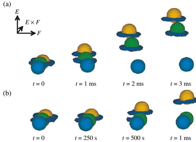
**Figure 4.** Demonstration of surface-sensitive particle separation. Particles with different anchoring strengths are dragged by an external force  $F = 6$  pN (a) and  $F = 20$  pN (b) in a nematic liquid crystal aligned such that  $E \perp F$ . The anchoring strengths of the blue, green, and red particles (bottom to top) are  $W = 1.5, 2.0,$  and  $2.5 \times 10^{-4} \text{ N m}^{-1}$ , respectively.
