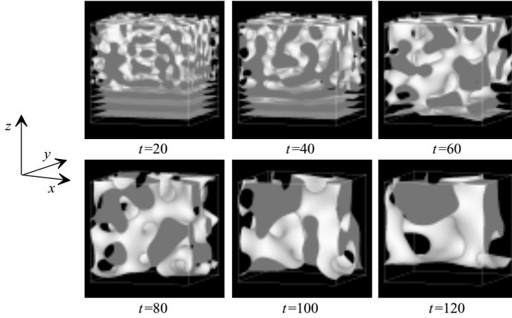
Fig. 1 – 3D pattern evolution during spinodal decomposition under the influence of wetting to the solid wall at the bottom ( $z = 0$ ). Here  $\Gamma = 10$  and  $\Xi = 1$ .
