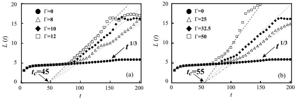
Fig. 3 – Temporal change in the thickness  $L$  of wetting layer for a solid ( $\Gamma = 0$ ) and fluid model ( $\Gamma \neq 0$ ). (a)  $\Xi = 1$ . The curves are  $L = 2.43 + 0.587t^{1/3}$  and  $L = 0.0120(\Gamma/\Xi)(t - t_c)$ ; (b)  $\Xi = 5$ . The curves are  $L = 2.43 + 0.587t^{1/3}$  and  $L = 0.0206(\Gamma/\Xi)(t - t_c)$ .
