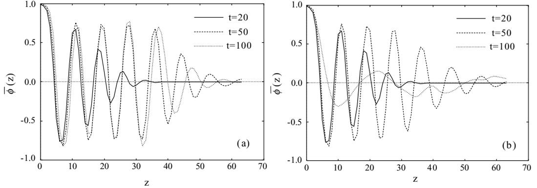
Fig. 2 – Temporal change in concentration profile along  $z$  (averaged over  $x$  and  $y$  directions),  $\bar{\phi}(z)$ , for (a) a solid model and (b) a fluid model ( $\Gamma = 10$  and  $\Xi = 1$ ).
