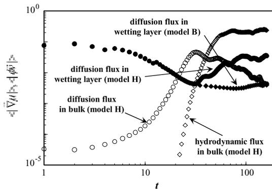
Fig. 5 – Temporal change in diffusion flux in the wetting layer and in bulk together with the growth of the hydrodynamic flux in bulk. Here  $\Gamma = 10$  and  $\Xi = 1$ .
