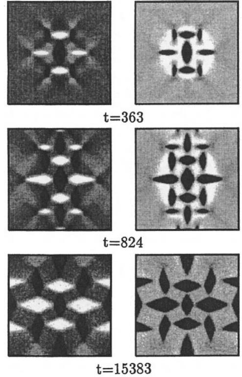
Fig. 1. Time evolution of  $\psi$  on the left and  $e_1$  on the right starting with a spherical droplet at  $t = 0$ . Elliptical domains (in black at  $\psi \sim 1.5$  and in white at  $\psi \sim -1.5$ ) are then successively created, while the gray regions remain in the disordered phase ( $\psi \sim 0$ ). Note that  $e_1$  is positive (in black) in the two variants of the tetragonal regions.
