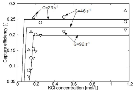
**Fig. 1** Capture efficiency vs. KCl concentration for  $2R = 1.96 \mu\text{m}$ : Symbols and lines are experimental values taken from Sato *et al.*<sup>1</sup> and theoretical ones based on trajectory analysis.
